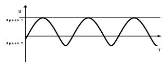
The rated voltage of the capacitor must be equal to or bigger than the highter one on the two Upeak1 and Upeak2.
